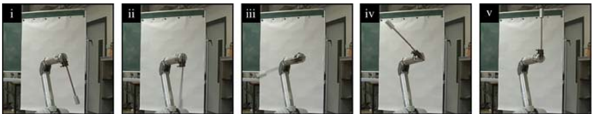
Figure 1.1: A robot manipulator swinging up to keep a heavy pendulum upright [2]
